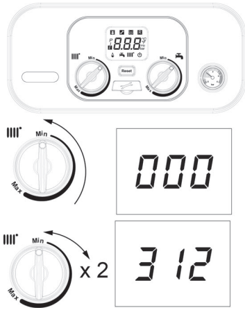
Fig.42 Setting de-aeration
